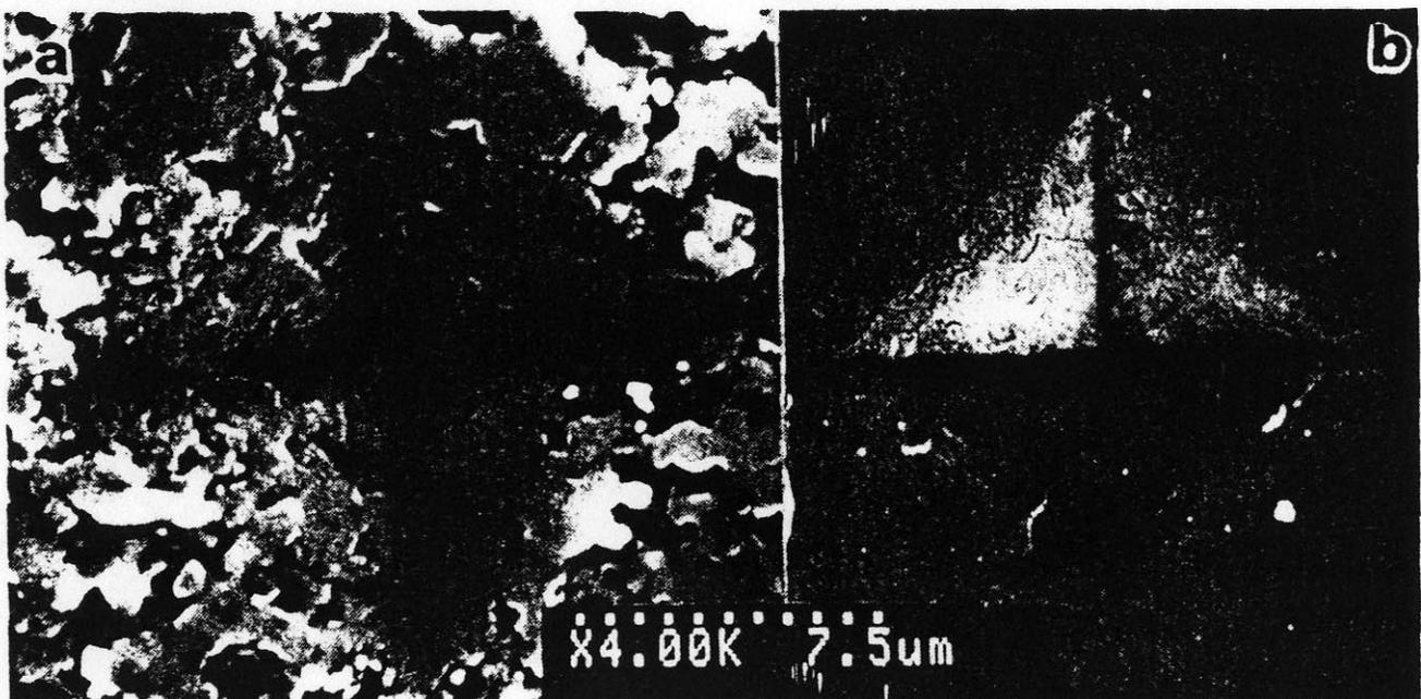
Figure 1: SEM micrographs of a) 1.19 N indentation in EB4 and b) a 1.73 N indentation in NT154.
