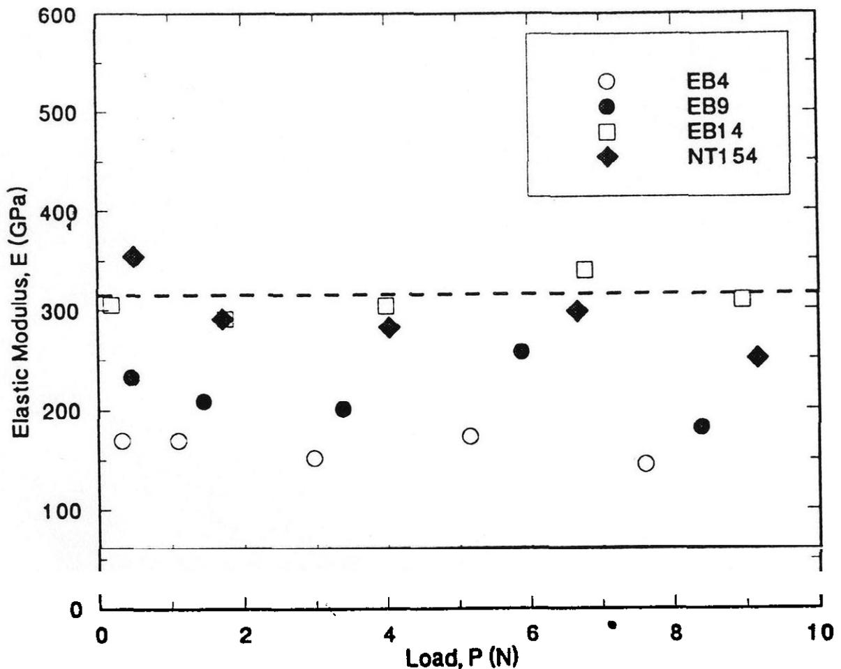
Figure 6: Elastic modulus vs. load calculated for four HIPed  $\text{Si}_3\text{N}_4$  materials using equation (4). Each point is the average of two readings. The dashed line represents  $E=315$  GPa as provided by Norton/TRW for NT154.
