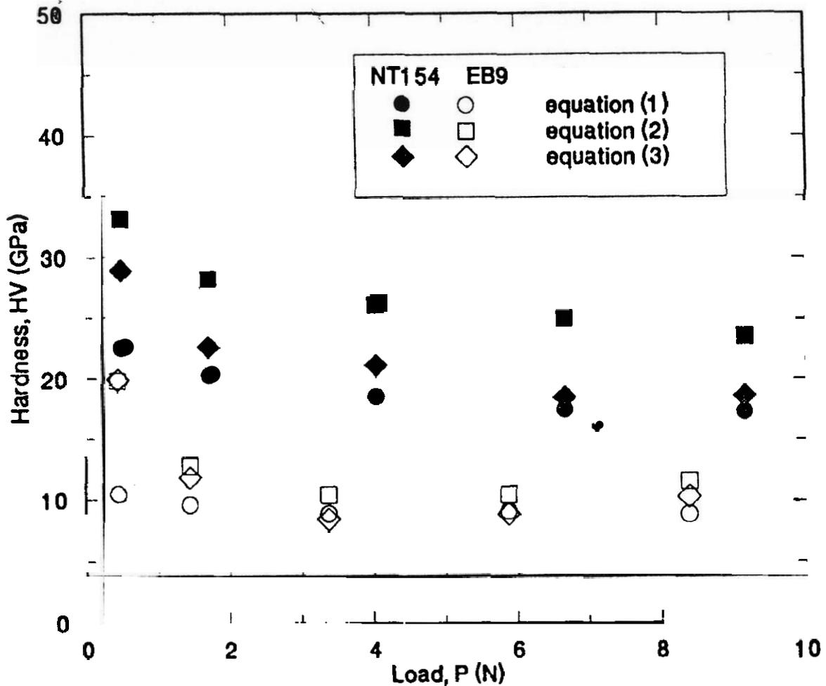
Figure 5: Hardness vs. load for specimens EB9 and NT154. Each point represents the average of two readings.
