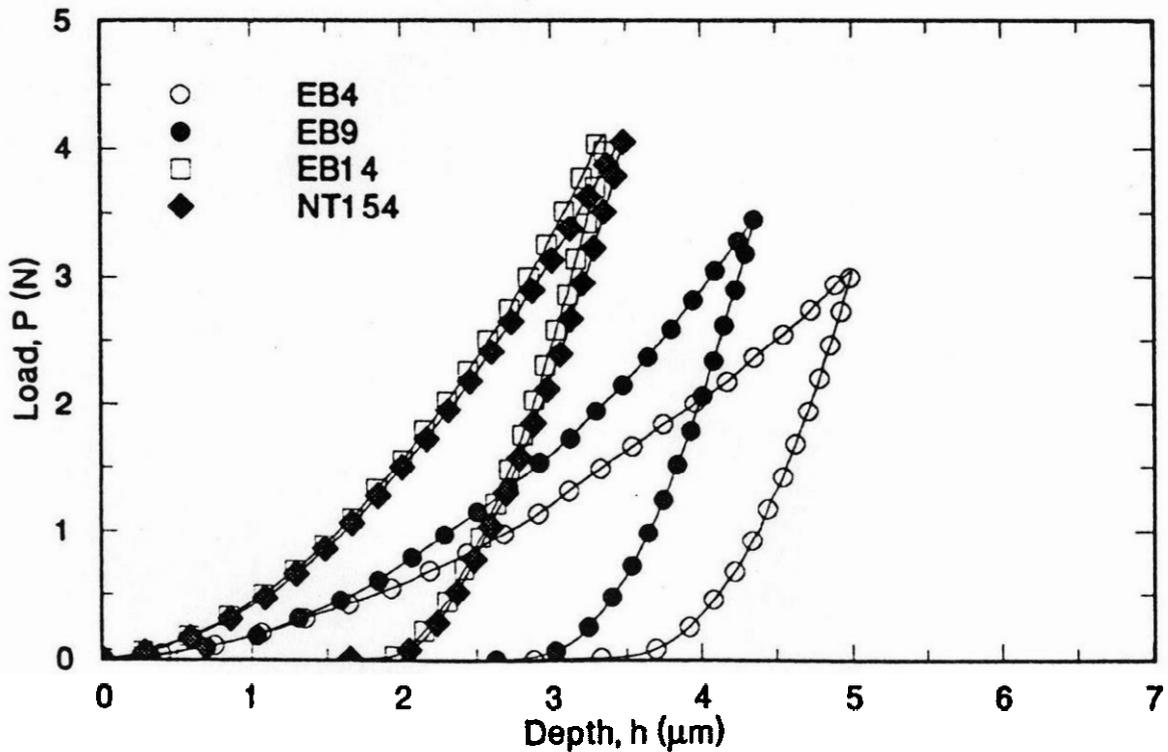
Figure 4: A comparison between load-depth plots obtained for samples EB4, EB9, EB14 and NT154 at the same total displacement.
