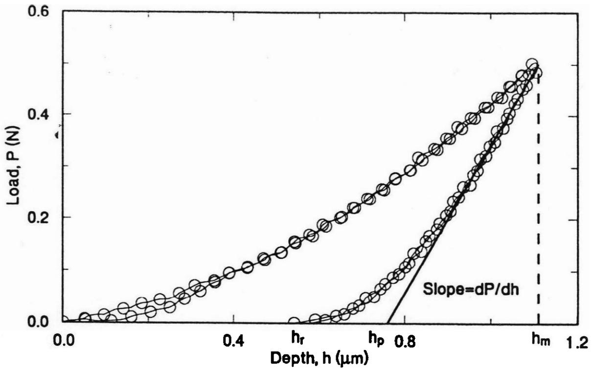
Figure 3: Two superimposed low load, load-depth plots for NT154.
