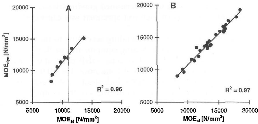
Fig. 2. Correlation between the modulus of elasticity (MOE) determined by the dynamic (vibration) approach and conventional bending method for sound beech (A) and spruce (B) specimens
