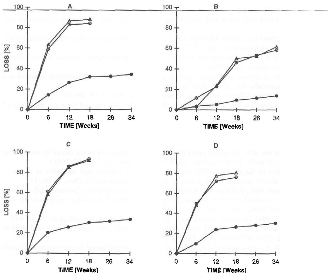
**Fig. 3.** The time course of wood decay in laboratory unsterile soil tests analysed by mass loss (-●-), MOE static (-▲-) and MOE dynamic (-○-). The wood species tested included: beech (A), keruing (B), poplar (C) and elm (D)
