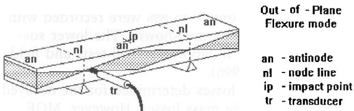
Fig. 1. Apparatus for measuring vibration parameters of rectangular wood specimens by free vibration
